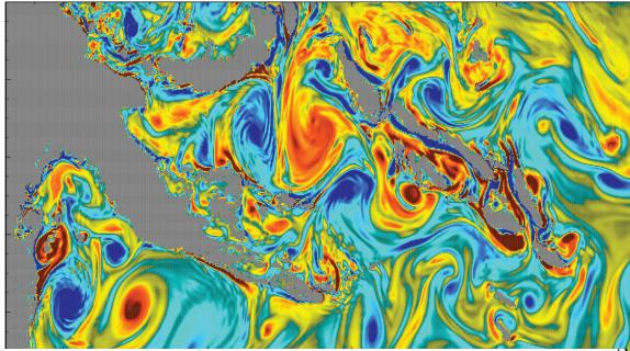
(right) The two-way AGRIF nesting system is used to refine the model resolution to  $1/36^{\circ}$  in a  $1/12^{\circ}$  global (Drakkar) simulation. From Djath et al 2014
